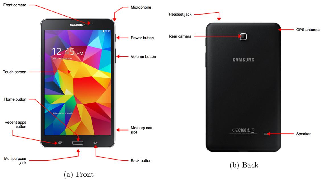
Figure A.1: Samsung SM-T230 device layout
